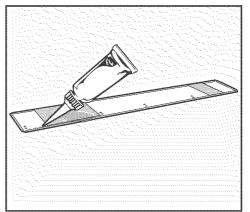
Squeeze the supplied silicone sealant along the groove of the deflector.
